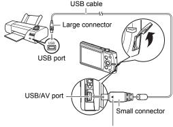
Making sure that the ◀ mark on the USB cable connector is towards the monitor screen side, connect the cable to the camera.
